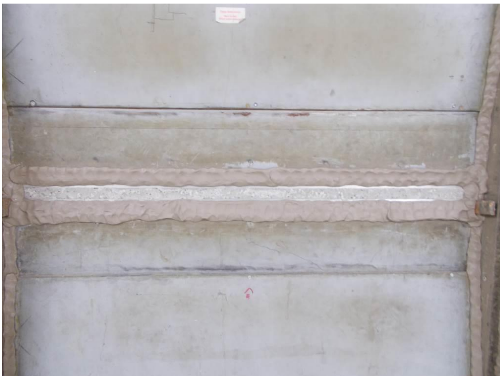
fig 3 Photo of the mounted element (with joint width of 30 mm, taken by ift Laboratory for Building Acoustics)
